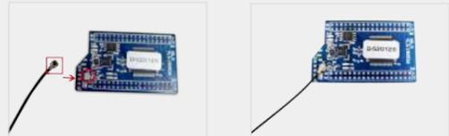
Stick the Wi-Fi antenna on the metal frame of UP BOX as shown in the picture below.
