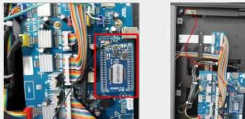
Put the jumper onto the 2 lower pins in the connector labelled "M-C", then install the back cover.
