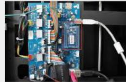
2\ Install the Wi-Fi enabled CPU for UP BOX.
