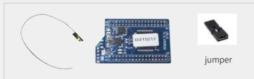
Connect the Wi-Fi antenna to the socket on the CPU.
