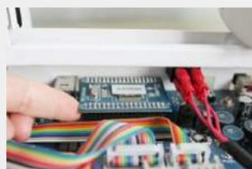
2\ Install the Wi-Fi enabled CPU.
