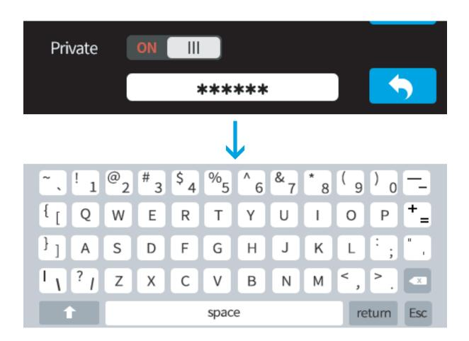
If user switches on the private function in WIFI setting, a password field will appear to allow password setup. This password will be required for WIFI connection to the printer to prevent unathorized usage through WIFI. Please note this is a weak protection that anyone who can access the printer through USB or touch screen could change the private password.
