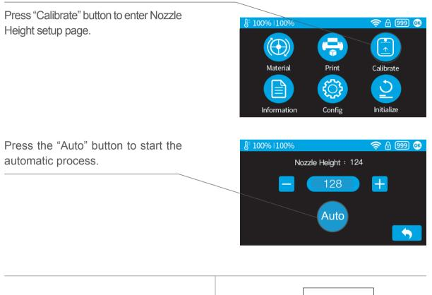
During nozzle height detection, the print head nozzle will touch the nozzle detector to make measurement.
