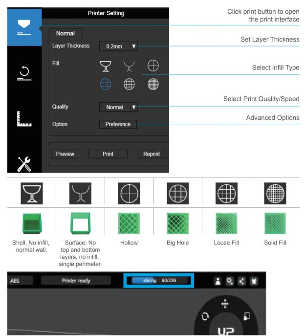
When the UP software is slicing or sending data to the printer, progress displayed on the status bar on top of the software interface. Do not unplug the USB cable as this will disrupt the data transfer and result in a print failure. The USB cable can be unplugged after the data transfer is finished.
