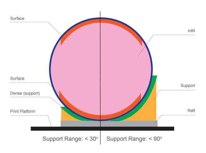
Dense: Solid support structure ensures that the surface being supported retains its shape and surface finish.
