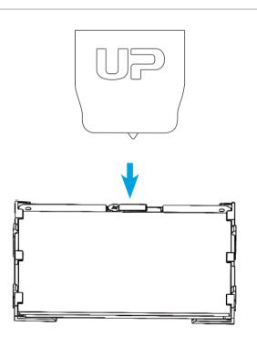
During nozzle height detection, the print head nozzle will touch the thin metal tab on the detector to make measurement.
