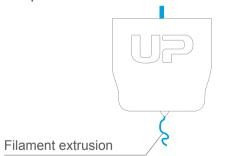
6\ Finally insert the guiding the tube in to the filament entrance and press the tube into the holding clip on the print head mount.
