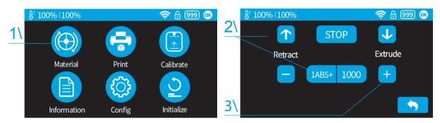
2 Choose the printing material as ABS by pressing the Wheel button to switch between different materials. Input the filament weight by using the +/- buttons.
