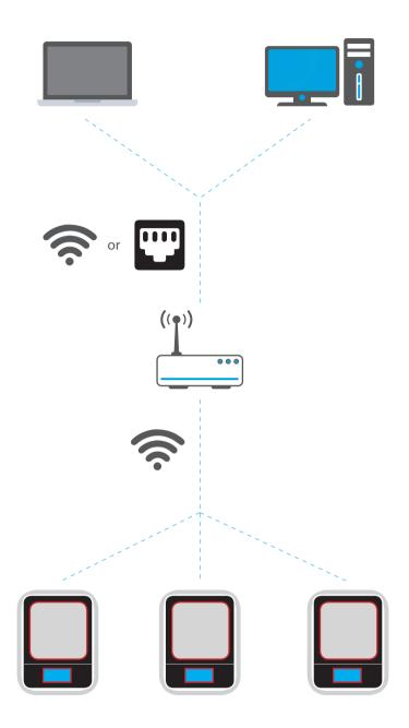
Connecting to the UP mini 2 through WIFI requires a Wireless Local Area Network (WLAN). Computer and printers must connect to the same WIFI network (same SSID) before able to communicate.
