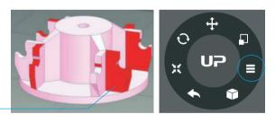
2\ Click the fix button the repair the model. The red defective surfaces will resume a normal color when repaired.
