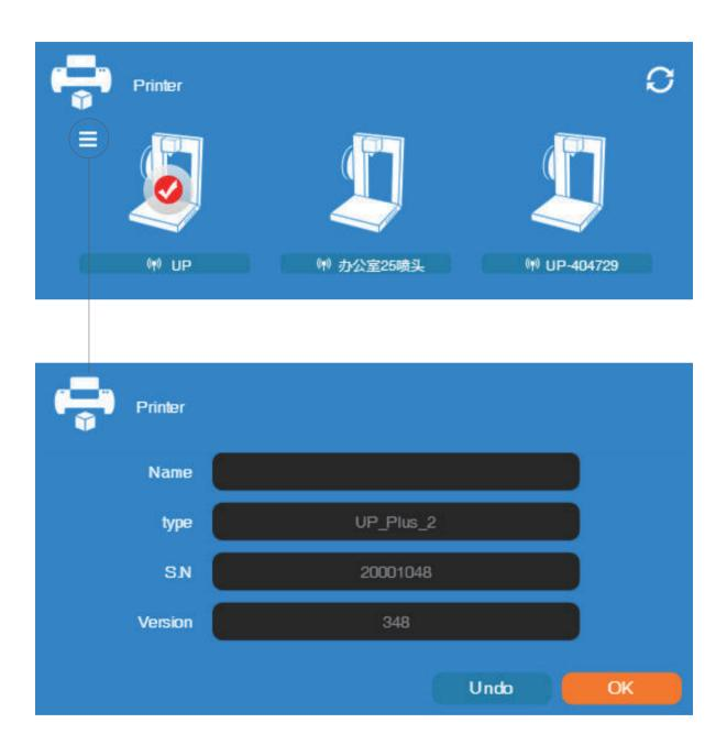
Printer info will be displayed by clicking the small button on the top left hand corner of the connected printer icon. Information including printer type, serial number and firmware version will be displayed. User could also set a custom name for the printer in the name field.
