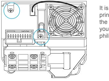
It is not necssary to remove the print head cover if order to remove the nozzle. However if you want to, you can do so by removing the two philip screws (circled).
