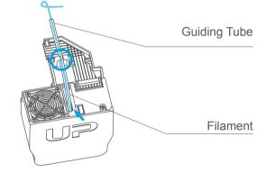
5 Check the nozzle for plastic extrusion. If plastic is coming out from the nozzle, that means the filament is loading correctly and the printer is ready for printing. (The extrusion will stop automat- ically.)
