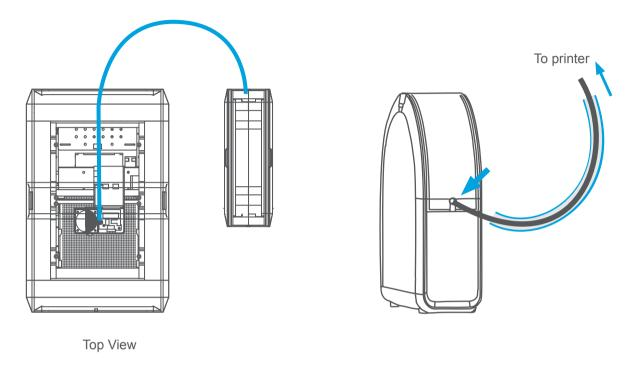
Push the guiding tube into the rubber ring as shown above.
