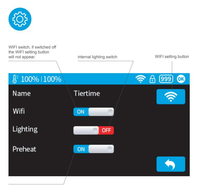
Preheat switch, when turned on, for every print job, the printer will first preheat 15min before proceed to printing.
